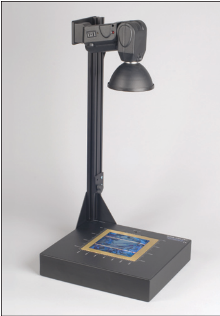
The Suns-Voc stage is available as an accessory to the WCT-120 lifetime testing instrument or as a stand-alone measurement system.
