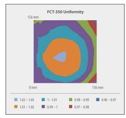
The uniformity of the FCT-350 is Class A  $(\pm 2\%)$  over 156 mm x 156 mm.
