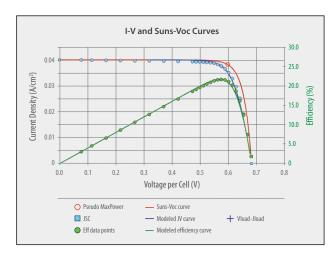
The instrument interface displays both 1-V and Suns-Voc data. This permits quick identification of shunt and series resistance effects.
